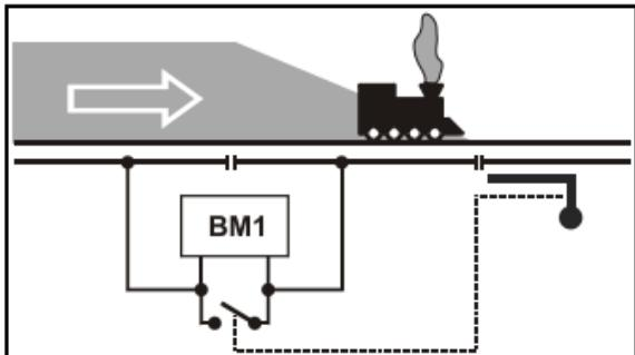
Technically, this is realised as follows: if the signal is "red", the BM1 module creates in the braking section an asymmetry in the otherwise symmetrical digital track voltage. This is spotted by decoders. The result is a gentle braking of the train until it comes to a halt, optionally with the set braking delay or set braking distance.
