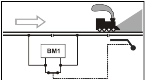
If the train is not to stop, but to continue unimpeded or to start moving again after the stopping time has elapsed, the BM1 will simply be bridged with a switch.
