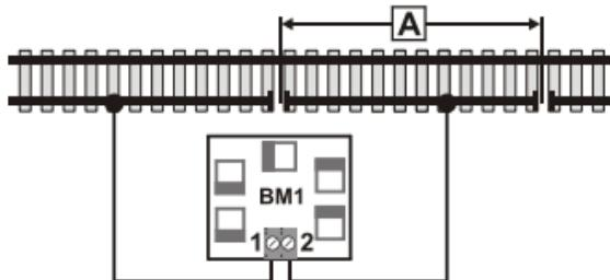
Use a switch parallel to the terminals 1 and 2 to switch the BM1 on or off. You can use a signal switch to do this. Most customary signals with double-coil drive are equipped with a switch like this.
